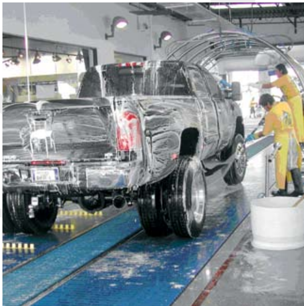
Rexnord® 6995 MatTop® Chain on AVW Transporter™ dual lane exterior car wash conveyor.
